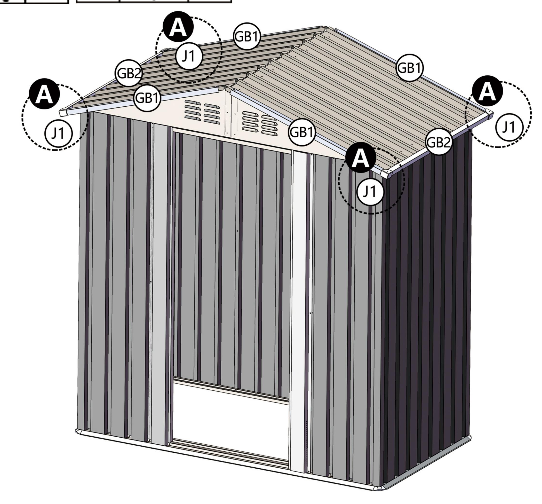
As shown in the picture, fix GB1 and GB2 with F1 on the edge, The four corners GB1, GB2, J1 share the hole position.
