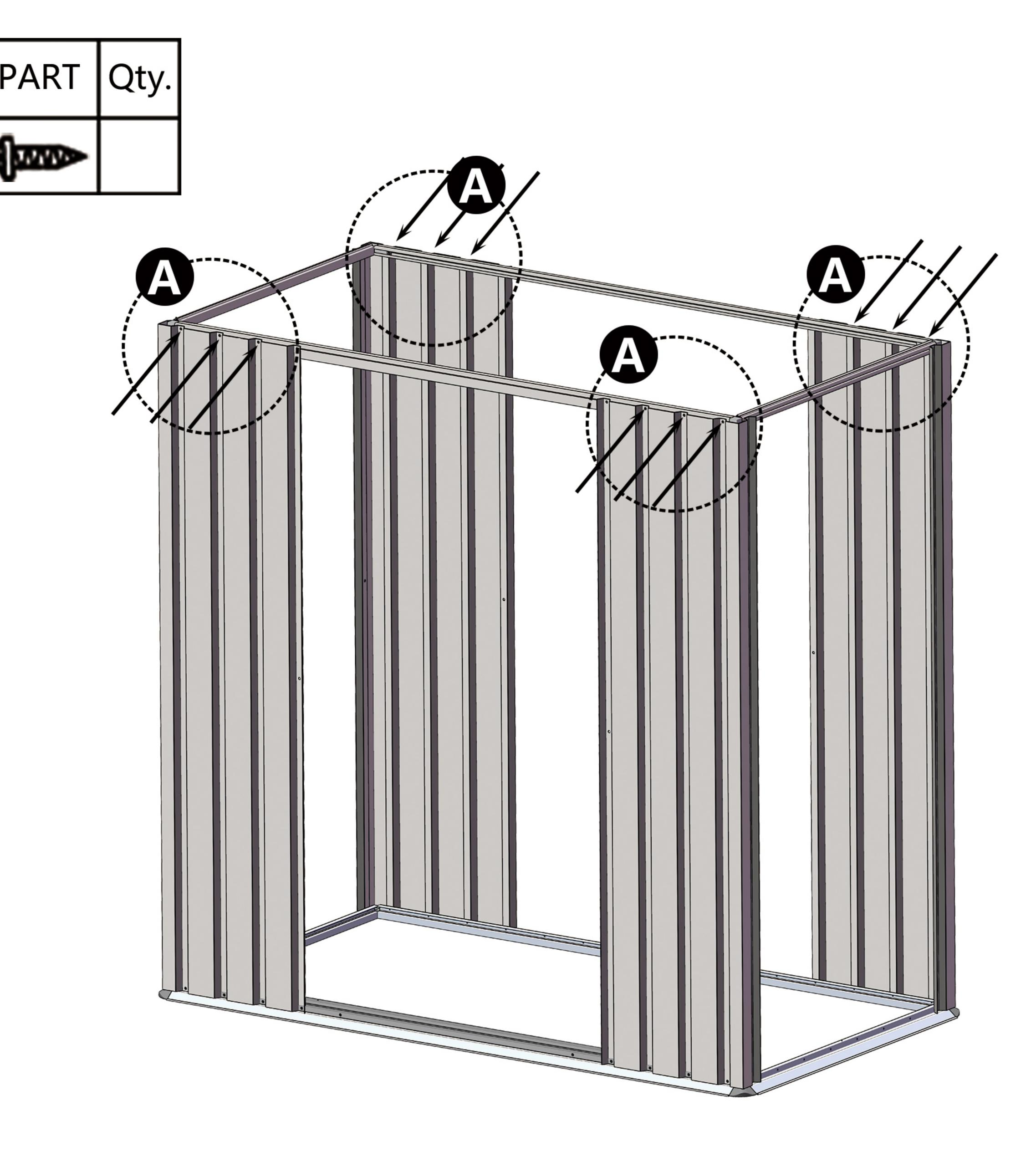
In this step, only the middle three holes need to be installed, and both sides need to be reserved.
