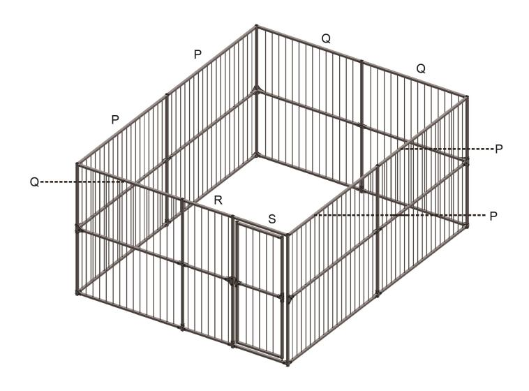
Gather(Quantity) (4)Corner Clamp (10)Gate Clamp (1)Gate Latch (18)Bolt and Nut
